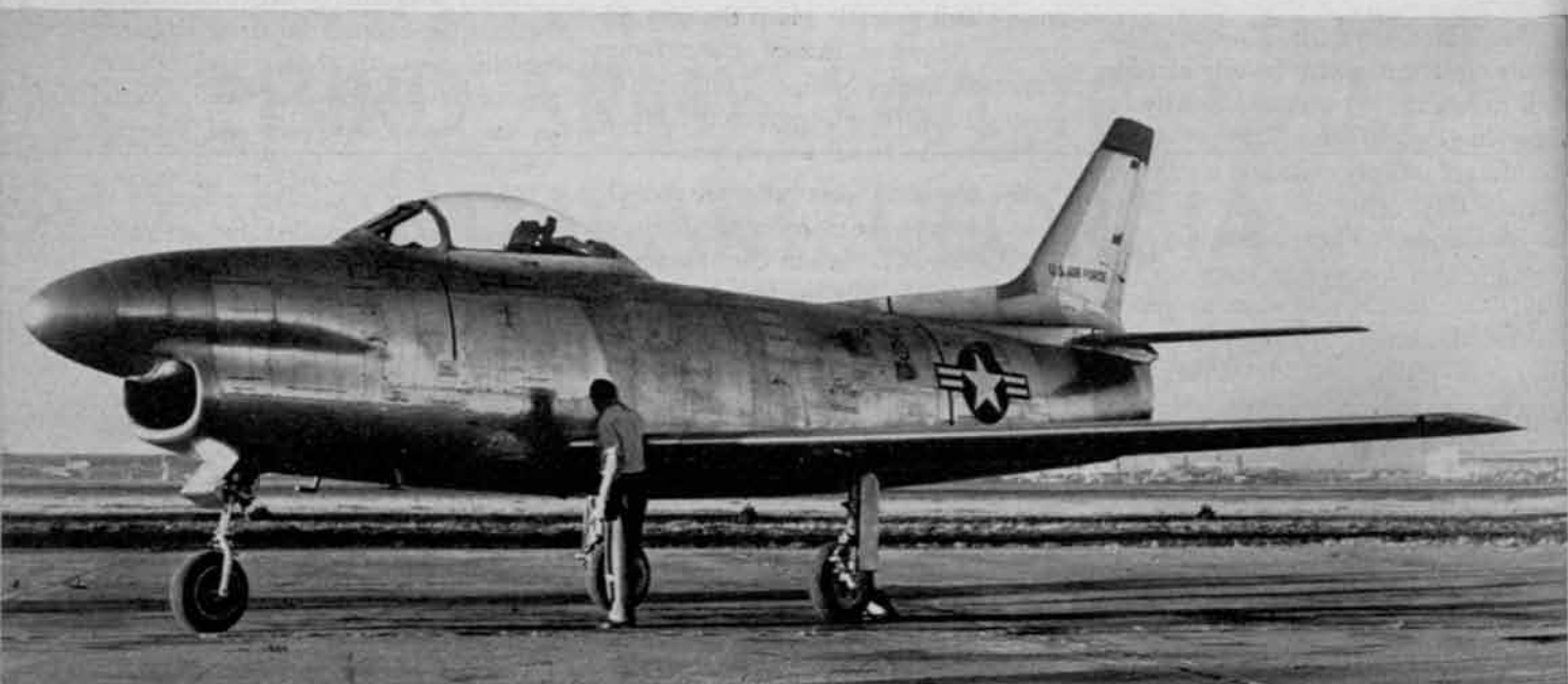
With speed of over 650 mph and a ceiling of 45,000 feet, the North American F-95-A is designed to climb quickly to extreme altitudes on intercept missions.
