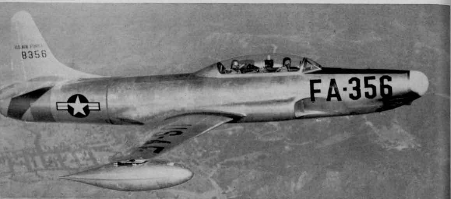
Lockheed's XF-94 is a modified version of the F-80 Shooting Star with a new electronic nose for night flying. In the 600 mph class, it is an all-weather fighter with a ceiling of over 40,000 feet.
