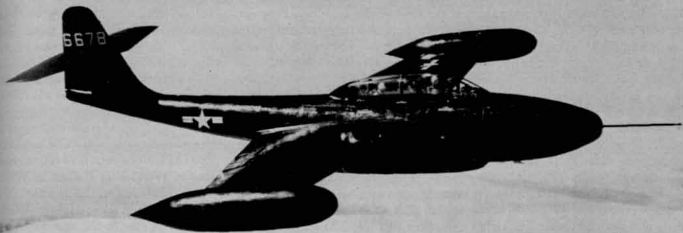
The XF-89, Northrop in the all-weather fighter family, has a speed and ceiling comparable to the XF-94. Its combat radius is over 600 miles.
