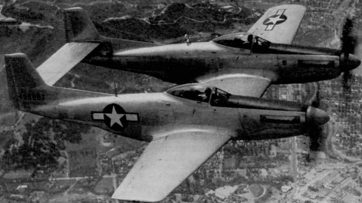
North American's Twin Mustang has a rate of climb of more than 5,000 feet a minute. It carries up to fourteen caliber .50 machine guns or eight MG's plus a supply of HVAR rockets.
